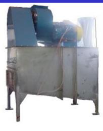
The compact scrubber uses a high velocity venturi (A) to create turbulent contact between the fumes/dust and the water.
